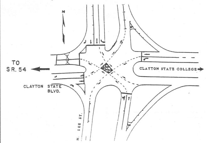
The new intersection at the entrance to campus is somewhat confusing until you get used to it. When this was designed, the engineers developed this concept because of the safety factors. This is a new innovation and is working very well, thus far. This map will hopefully make it easier for the student body, faculty and staff to understand this new concept.
